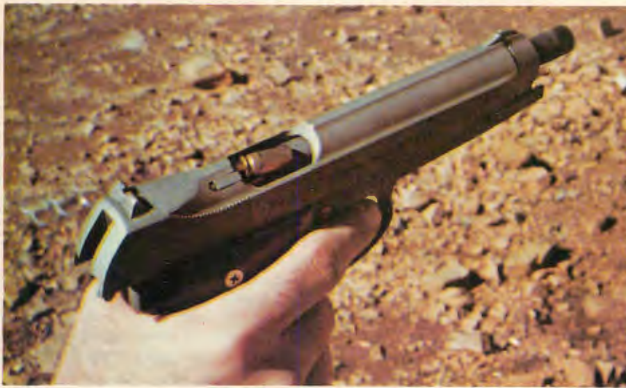
Above: Failure to eject.
